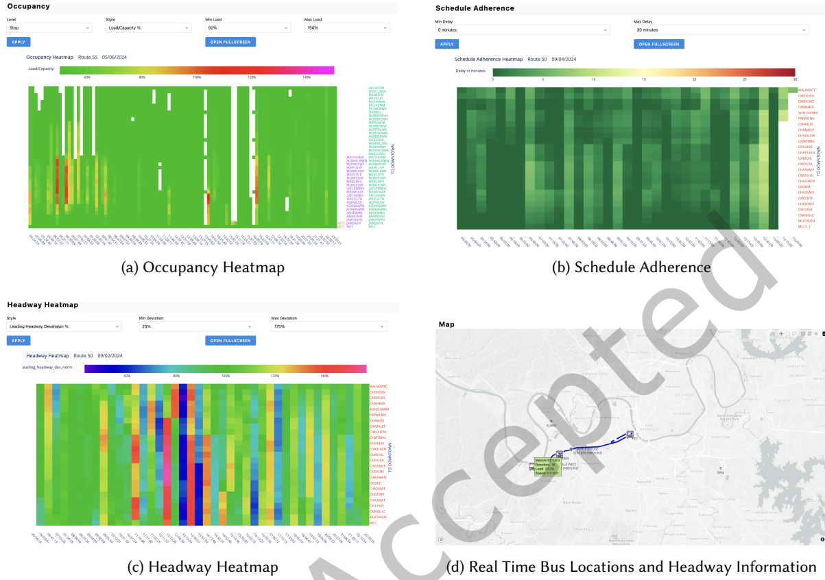
Fig. 8. Other visualizations offered on Vectura. Aside from the real time bus locations, all other plots are available for both historical and real time data. Similar to the string plots, these plots provide information for a specific aspect of different routes, at a glance.
