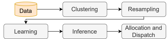
Fig. 2. Overview of our incident prediction approach. We extract spatial temporal information from a variety of data sources, focus on heterogeneity not explicitly modeled in the feature space by identifying clusters, perform resampling to address sparsity, and learn models on incident occurrence.
