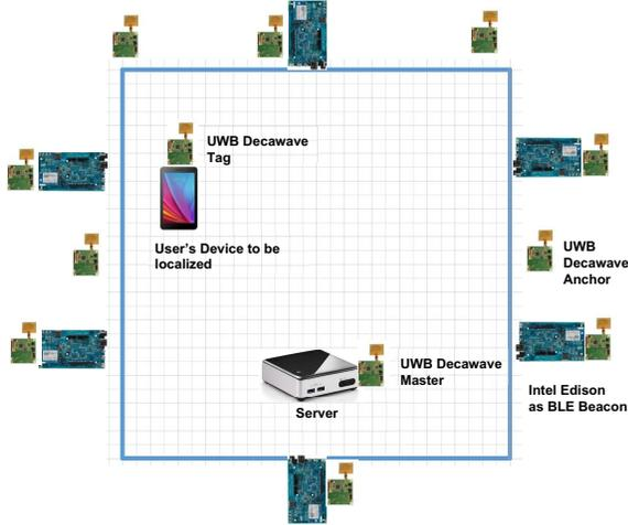
Fig. 2. Indoor localization experiment setup with 6 Intel Edison boards acting as BLE beacons; 12 UWB Decawave sensors; centralized server for sensor processing and the android tablet whose position is to be localized.
