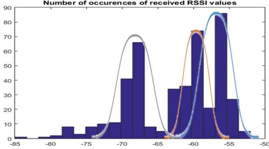
Fig. 1. A representative histogram of RSSI values received from a beacon. The three peaks correspond to the mean RSSI value received on each of the three advertising channels. Though the association between beacon messages and the corresponding channels is not available through the Android BLE API, by modeling the histogram as a mixture of three Gaussian kernels, the mean and variance of the RSSI values can be estimated on a per-channel basis.
