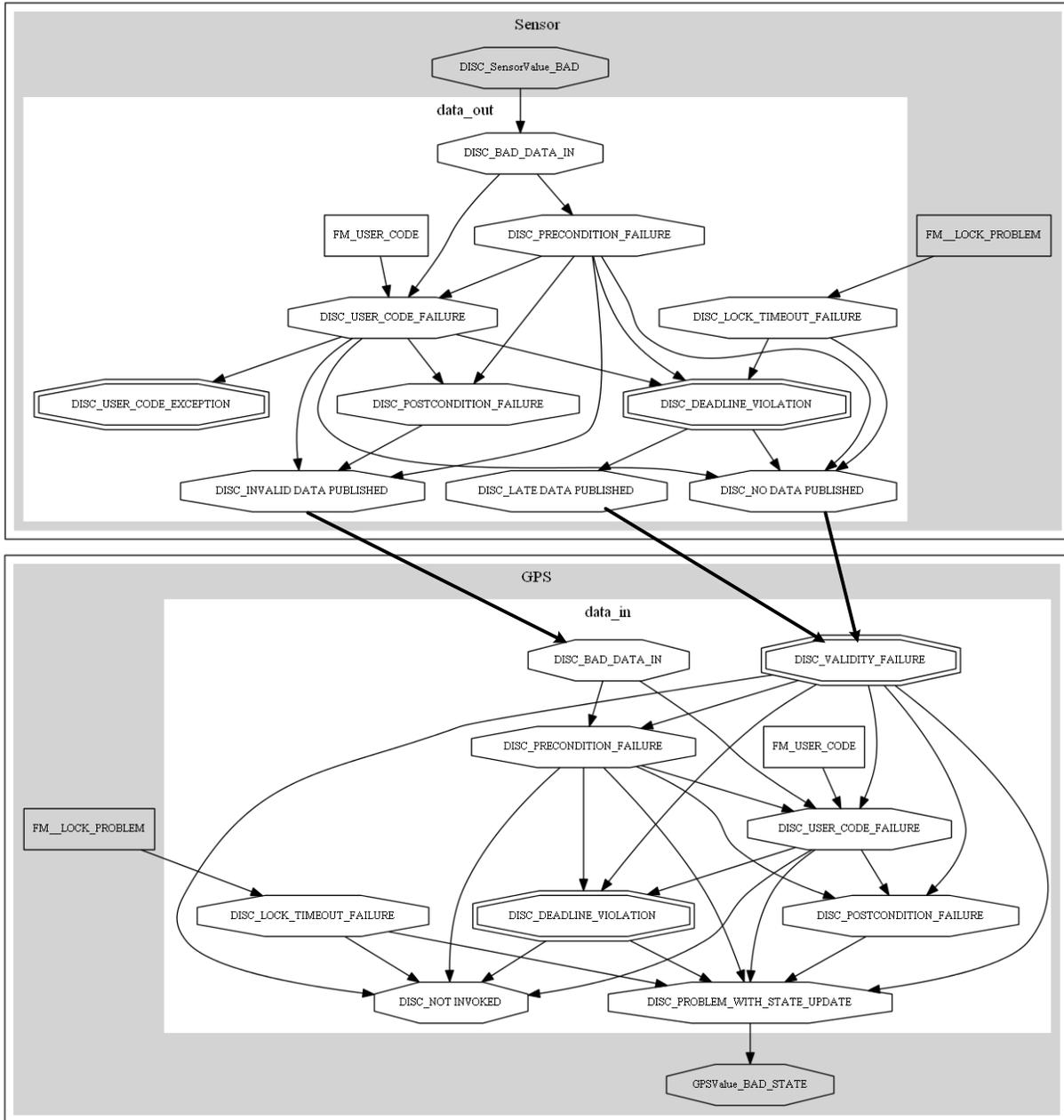
Fig. 5. TFPG model for Sensor-Publisher and GPS-subscriber
