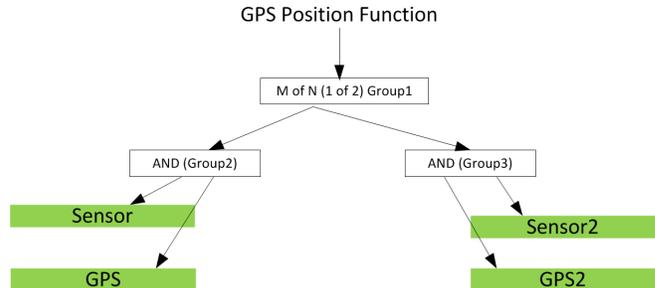
Figure 4. Example showing allocation of the GPS position function shown in Figure 3 to the components shown in assembly of Figure 1.
