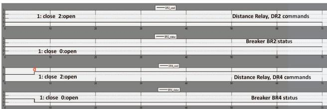
Fig. 9. Distance relay commands and breaker status for scenario 2
